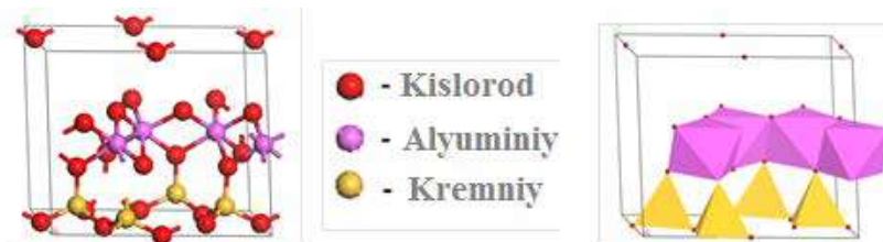
3-rasm. Kaolinitning ( \text{Al}_2\text{Si}_2\text{O}_9\text{H}_4 ) kristall strukturasi
